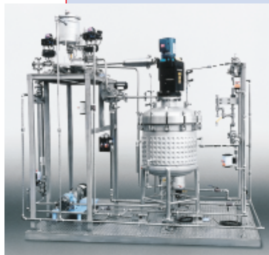
Skid mounted 180 liter reactor/liquid distribution system. Includes automated dosing vessel, load cells, heat exchangers, temperature controls, and filters. Completely stainless steel.
