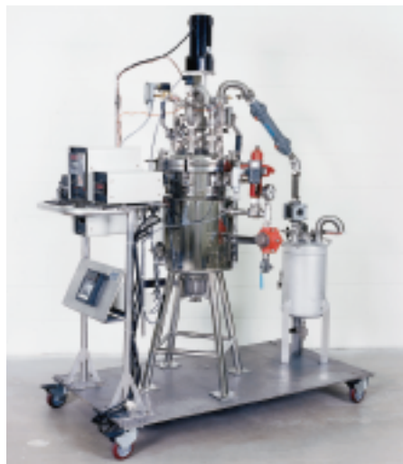
Reactor/Evaporator for foods and flavors processing. Equipped with pH and steam heating/water cooling controls, recorder, condenser, and receiver.
