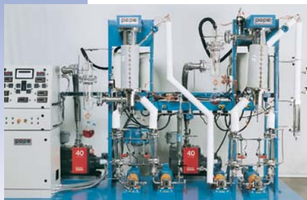
Turnkey, 6', two-stage Molecular Still Pilot Plant for long chain ester purification
