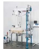
4-gallon, 2" diameter, high vacuum and high temperature Fractional Still for fine chemicals manufacturing
